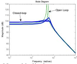
Fig.9 Open- and closed-loop frequency responses
