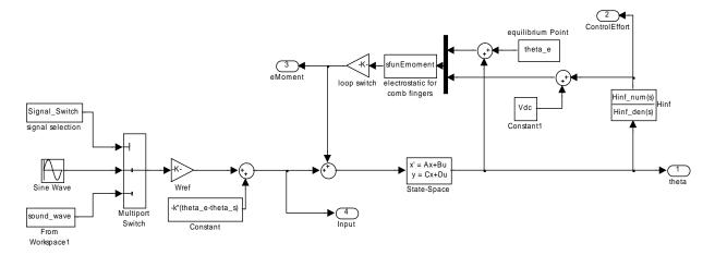
Fig.10 Simulink diagram of the closed-loop microphone
