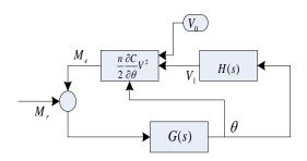
Fig. 2 A proposed active damping configuration
