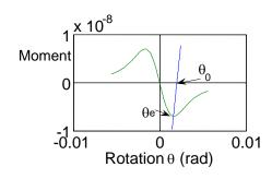
Fig. 4 Graphical solution of  $\theta_e$  when the initial unforced rotation is  $\theta_0$  with a DC bias of 0.1 V
